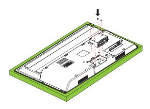
**3** Secure the stand to the stand column using the five long screws (provided).
